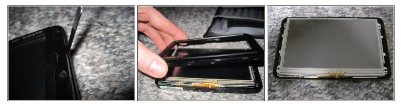
Now to pry screen retainer away from the back Plastic/Rubber side. To pry away take pry stick straight down between retainer and plastic/rubber back side and begin to pry up. If it doesn't come undone, pry in different spots little by little and it will come undone.
