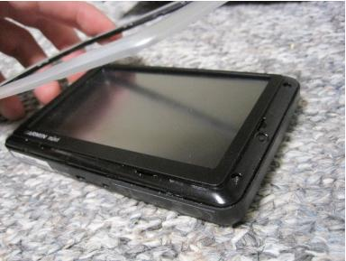
First you pop off the silver retainer around the whole gps system. The retainer is snapped on in various spots all around the retainer. Just work your way around till you pop all the snaps and it will come right off. Take not of the hole you see on the left part of the screen on the retainer to put back on the right way.
