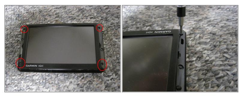
Now you need to take the 4 screws that are cicled in red out using a T5 Torx bit found in the protool kit.
