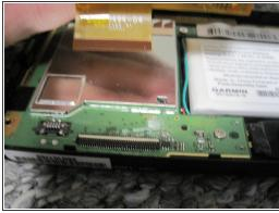
• As you life the screen up off the circuit board there will be a ribbon cable attaching the screen to the board. Take a plastic tool on the top side of the white connector and pry up on it to disconnect the ribbon cable.
