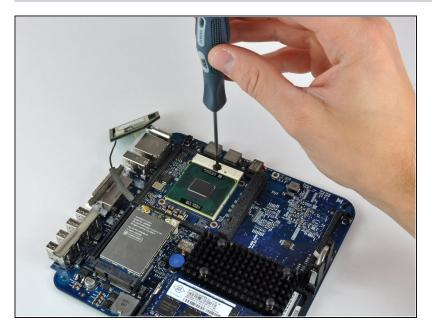
Use a small flathead screwdriver to rotate the processor lock 180 degrees clockwise until the indicator points toward the closed lock symbol.
