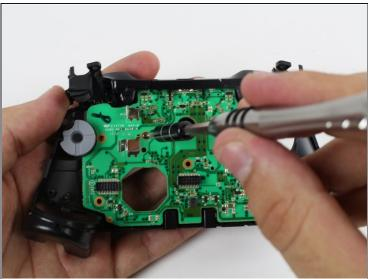
Remove the six T6 Torx screws located on the bottom motherboard.
