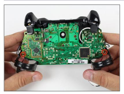
Unscrew the two 7mm T6 screws located near the rumble motor sockets.
