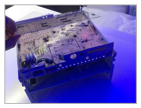
The chassis and the power supply board were cleaned up and adapted for fitting the new components.
