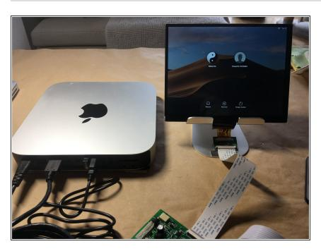
Testing the new HDMI 8" LCD screen.
