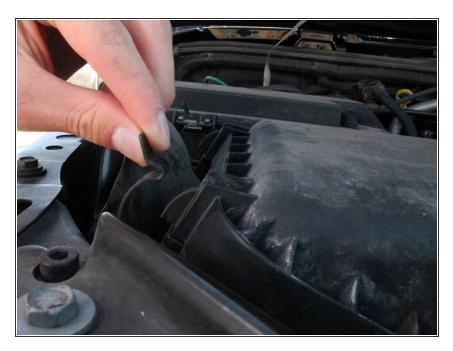
To unlock the air filter box, grasp each clip and pull the clip away from the air filter box.
