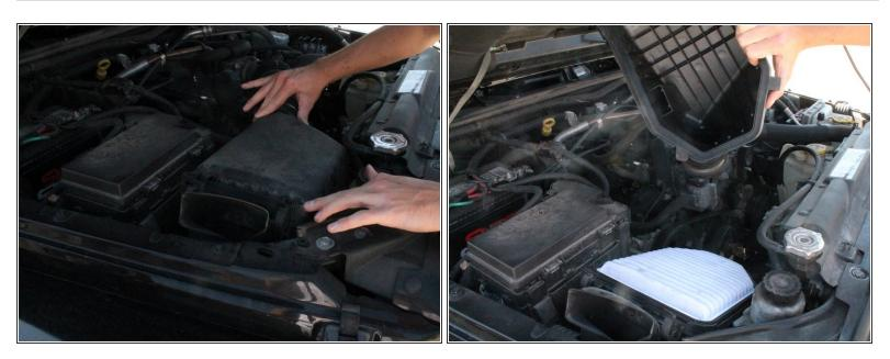
After you have removed the 4 clips, carefully pull and twist the cover off. You now have access to the air filter.
