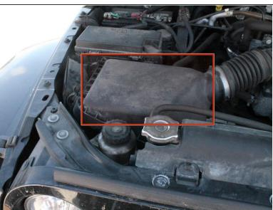
Locate the air filter box in front of the car battery. It will have a 4-inch diameter hose coming out of one side (towards the center of the vehicle) and an air release coming out of the other side. It should have four clamps keeping it sealed.
