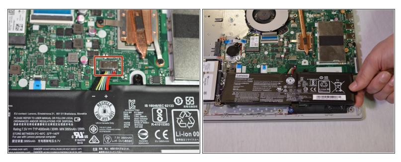
Disconnect the battery connector by pulling toward the battery parallel to the motherboard.
