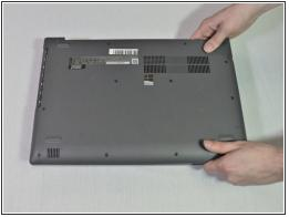
Use an opening tool to pry out the back cover.
