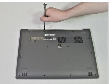
Using the Phillips #1 screwdriver, remove the twelve screws around the back panel from the laptop.
