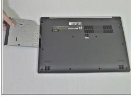
Carefully remove the optical drive bracket by pulling the bezel away from the laptop.
