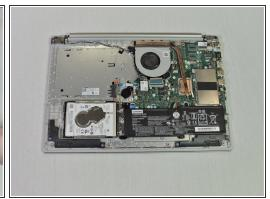
Remove the back panel by pulling it up and away from the laptop.
