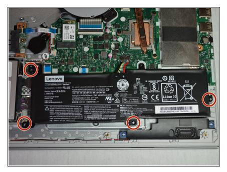
Remove the four 6mm screws using the Phillips #1 screwdriver.
