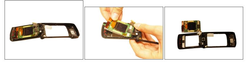
Hold the outer phone casing and pull the LCD screen out.
