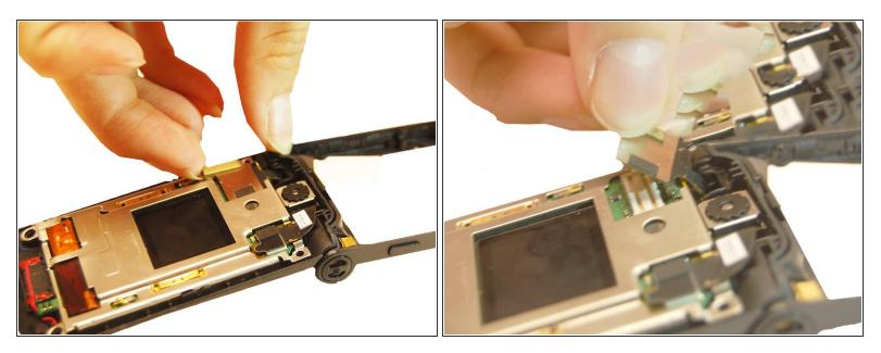
• Pull the flex cable connection away from the top of the phone.
