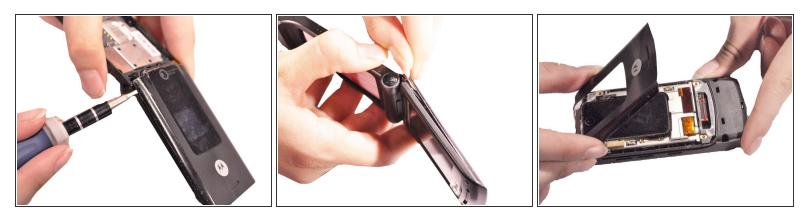
• Use a flathead screwdriver or plastic opening tools to help pry the top cover away from the phone.
