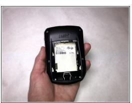
Remove the battery from the compartment.
