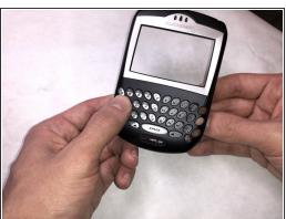
Push the keyboard from the front view to separate it from the front housing.
