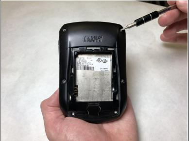
Remove the four 10.7 mm Torx T6 screws.
