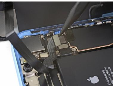
Use the tip of a spudger to pry the front sensor assembly connector up from its socket.
