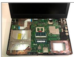
Remove the ribbon connectors that connect the keyboard to the motherboard. The keyboard should now be completely disconnected from the laptop.
