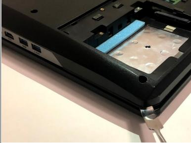
Begin to pry the keyboard off of the laptop with the pointed metal spudger.
