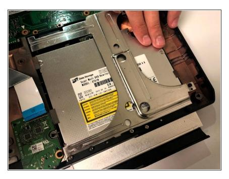
Placing your hand on the side of the disk drive closest to the motherboard, slightly push down and out to remove the drive.
