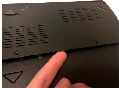
• Find the panel on the back of the computer. Use a Phillips #0 screwdriver to unscrew the 2 4.2mm screws on that panel. Next, lift up the panel at the indent and place it aside.
