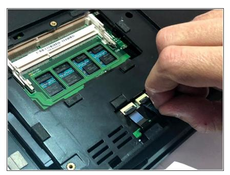
When the back panel is removed, disconnect the blue and black ribbon connectors exposed from the back panel.
