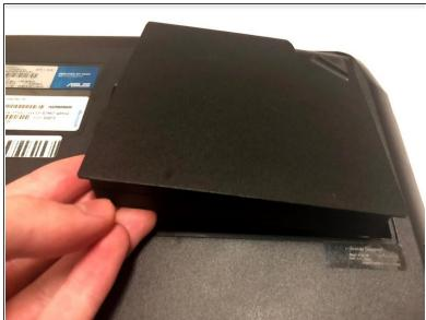
Make sure the computer is off and turn it over on its back. Push the slider all the way back until the compartment for the battery opens. Remove the battery and place it aside.
