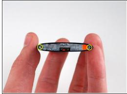
No surprises here. This design is identical to the 4th Gen nano. Even though the exterior hold switch is near the edge of the iPod, the internal hold switch is actually in the center of the iPod.
