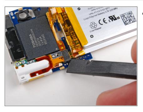
Removing the connector that connects the microphone, speaker, hold switch, and headphone jack to the logic board.
