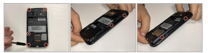
Using a Phillips #00 screwdriver, remove the screws as directed.
