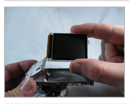
The LCD has been removed! It can now be replaced with a functioning display.
