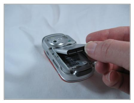
Lift battery at the rounded notch near the bottom of the phone.
