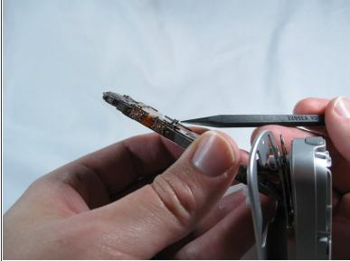
• The LCD display is connected to the device with a small flex cable. To release the cable, flip the small handle on the connector to an upright position.
