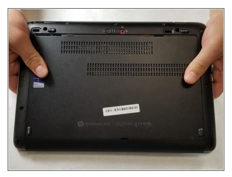
• Slide the back cover plate forward to remove it.
