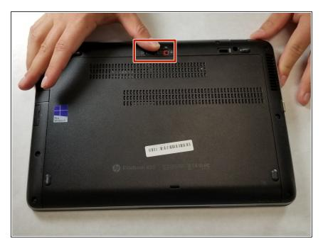
• Slide the latch to unlock the back cover.
