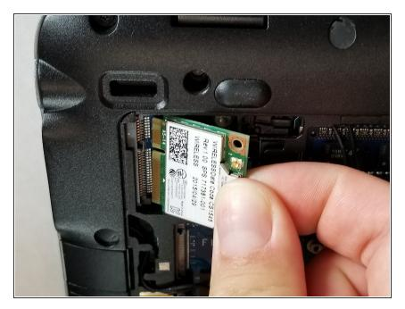
• Pull back the Wi-Fi card and lift up to remove it.
