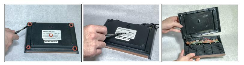
Using the screwdriver and the PH1 bit, unscrew the five 10.0 mm screws on the bottom of the console.
