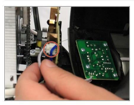
Once the housing has been pulled upwards, carefully uplug the wire connecting the browning dial circuit board to the main circuit board.
