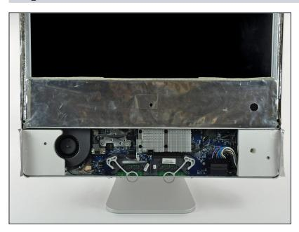
• Tape the lower EMI shield up against the face of the display to keep it out of the way while you work.
