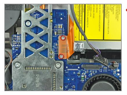
• Remove the two T6 Torx screws securing the optical drive connector to the logic board.
