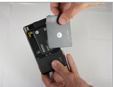
Place thumb on the back cover, and push down towards the bottom of the device. Once the cover releases, pull it away from the phone and set it aside.
