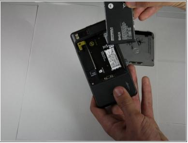
Find the yellow pull tab located in the upper left corner. Pull the tab until the battery dislodges.
