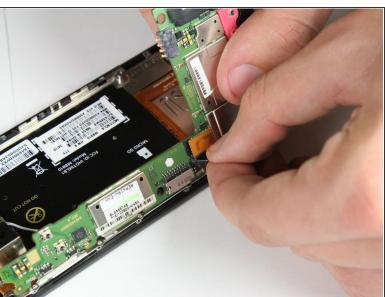
Scrape away the electrical tape that covers the LCD and digitizer cable using the spudger tool or a fingernail.
