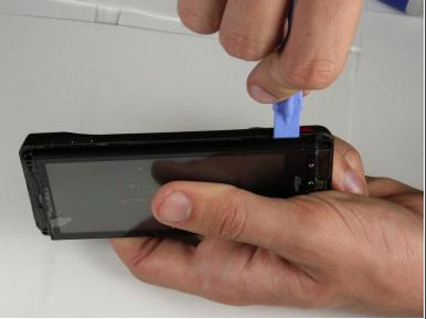
Locate the seam along the right edge of the phone. Use the prying tool to disconnect the two clips along the edge.
