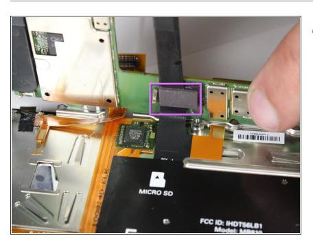
Using the spudger tool, pop the black cable connector off of the motherboard.
