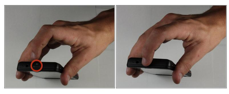
Locate the power button at the top of the phone. Depress power button for 2 seconds until a menu appears.
