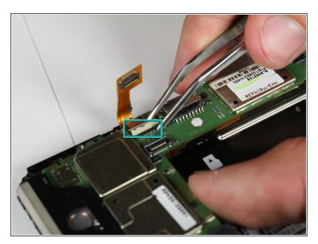
Carefully flip the small white connector up and away from the motherboard.
