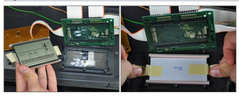
• Replace the LCD screen and tape it down to the top cover.
