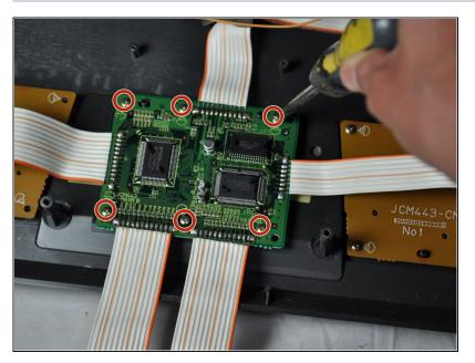
Completely unscrew and remove all six of the screws on the central circuit board.
