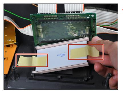
Remove tape from the LCD screen and remove the screen completely.
