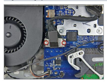
Remove the two T6 Torx screws securing the display data cable connector to the logic board.
