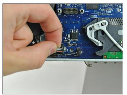
Disconnect the hard drive fan by pulling its connector away from the face of the logic board.
