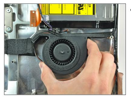
Lift the optical drive fan off the plastic posts protruding from the rear case.
