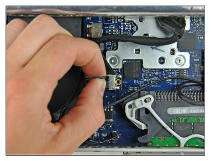
To disconnect the display data cable, grab its connector's black tab and pull it away from the face of the logic board.
