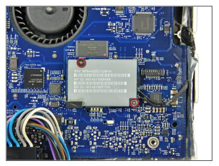
Remove the two Phillips or two T6 Torx screws securing the AirPort/Bluetooth board to the logic board.
