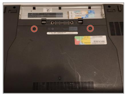
• Remove two Phillips head screws from the bottom cover.
