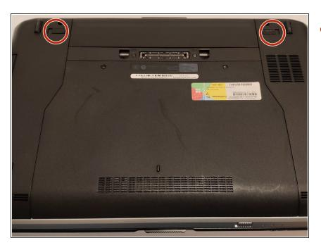
• Slide the two notches outward. Lift the battery outward and pull.
