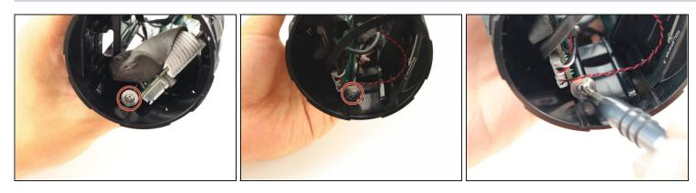
• Remove the two 9mm Phillips #1 screws holding in the sides of the motherboard.
