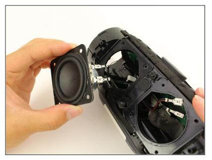
Now that the second speaker is disconnected from the motherboard, pull the speaker and wires out of the housing.
