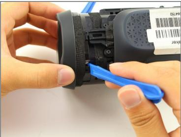
• Insert the plastic opening tools underneath both tabs.
