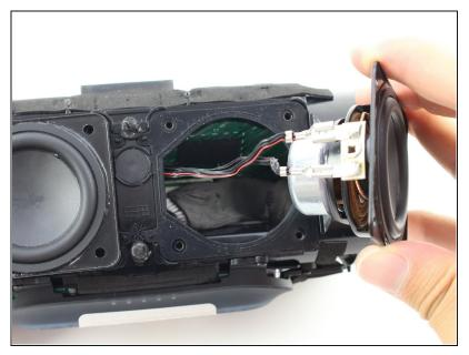
Pull gently on one of the speakers so it is outside of the housing. Be careful as it is still attached with the wires to the motherboard.
