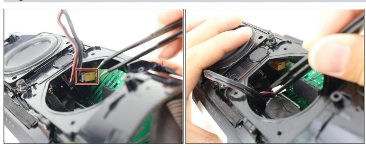
• Grab the bundled cable connector that joins the speakers to the motherboard with <u>tweezers</u>. Gently pull the connector free.
