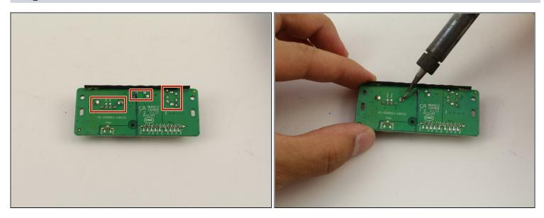
• Desolder the USB, MicroUSB, or AUX port off of the circuit board.
