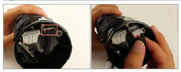
Pull gently to disconnect the bundled cable connector in the side of the speaker. This
