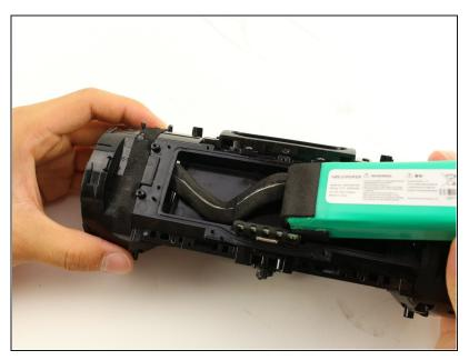
• Pull the battery and battery cable out from their housing.
