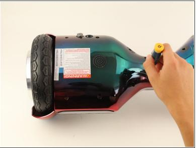
Remove the two 11mm Phillips #1 screws that hold the base plate to the body.
