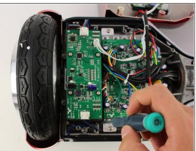
Remove the four 11mm Phillips #1 screws that hold the cover on.
