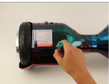
Remove the six 12mm Phillips #2 screws holding the base plate.
