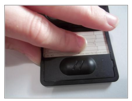
Loosen the plastic contact list covering by sliding it to the left.
