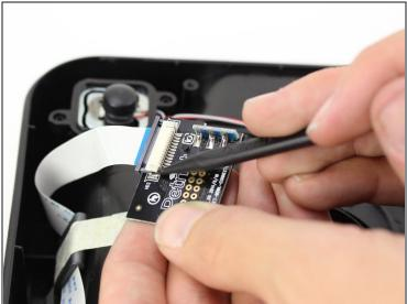
• Push the small gray pieces on the ribbon connector into the "open" position with the nylon spudger.
