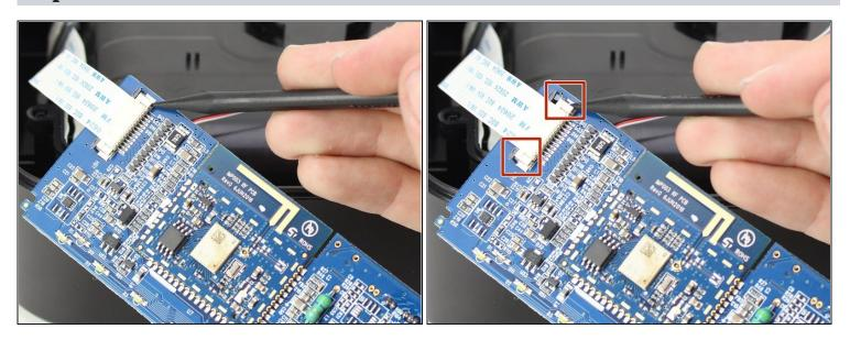
• Push both small gray pieces next to the ribbon connector towards the ribbon to put them in the "open" position using the nylon spudger.
