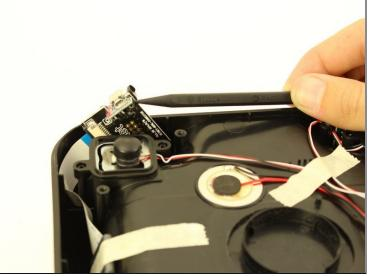
• Use the nylon spudger to remove the charging assembly from the SmartBowl.
