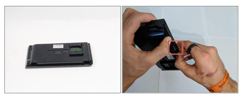
• Remove the back cover from the display assembly by pressing down on the point of connection.
