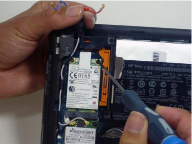
Use a Phillips #00 screwdriver to remove the two Phillips 2.0 and 3.0 mm screws that secure the WWAN to the system board.
