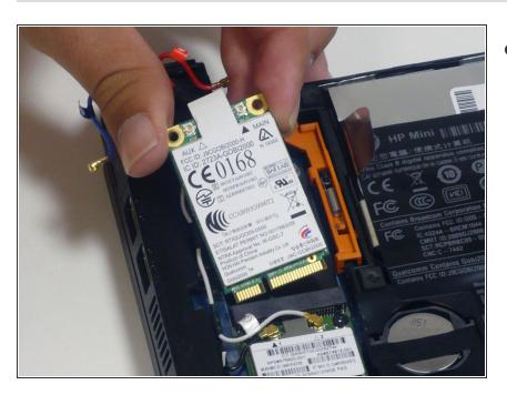
Remove the WWAN card by pulling the WWAN card out at an angle.
