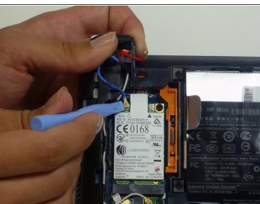
Disconnect the two gold antenna cables from the WWAN card using a plastic opening tool.
