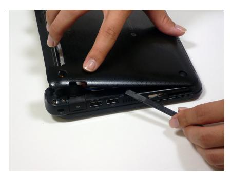
Use the spudger to pry off the back case by the edge near the battery compartment, and work your way to the sides. The case will then pivot along the front edge.
