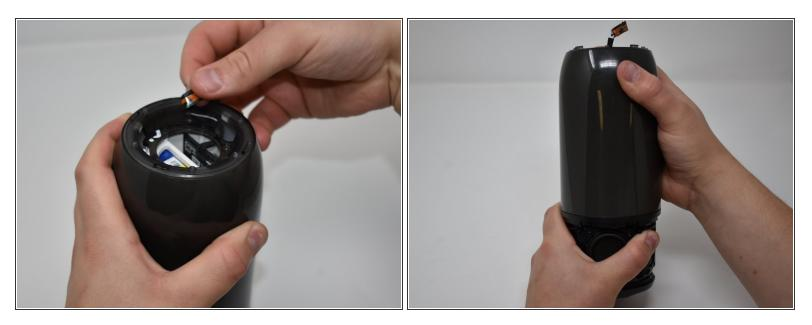
Peel off black, taped-on electrical lead from the inside side of the JBL Pulse 3.
