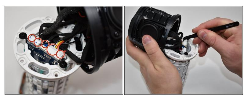
• Use tweezers to pull the five connections off of the LED light display.
