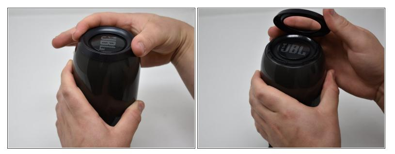
• Turn the JBL Pulse 3 right-side up and unscrew the top ring of the device. A small amount of force and/or a cotton cloth may be necessary to remove this piece.
