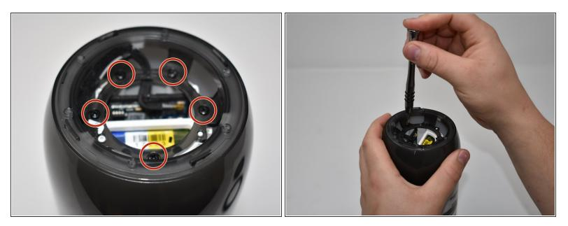
• Remove the five 7mm screws on the inside of the JBL Pulse 3 with a Phillips #1 screwdriver.
