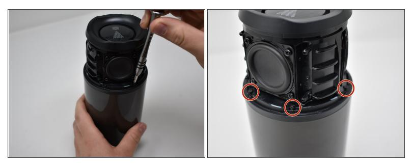
Use a Phillips #00 screwdriver to remove the six black 6mm screws on the inside of the top of the bottom section.
