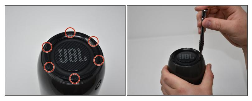
• Remove the six 5mm screws on top of the JBL Pulse 3 with a Phillips #0 screwdriver.
