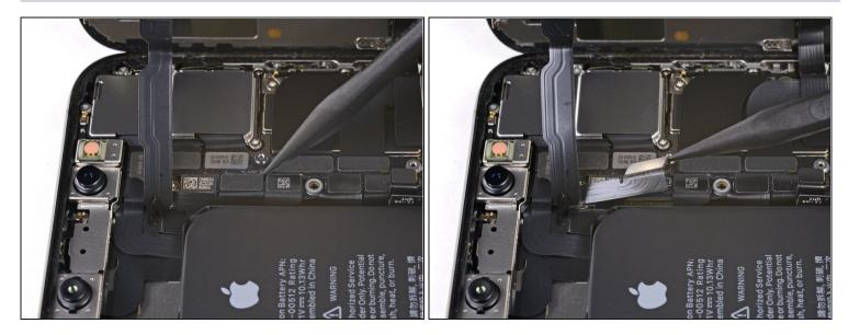
• Use a spudger or a fingernail to pry up and disconnect the front panel sensor assembly connector.
