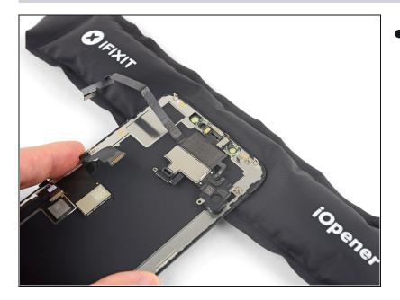
• Use a hairdryer or heat gun or prepare an iOpener and apply it to the top front of the display for about a minute, in order to soften the adhesive securing the sensors.
