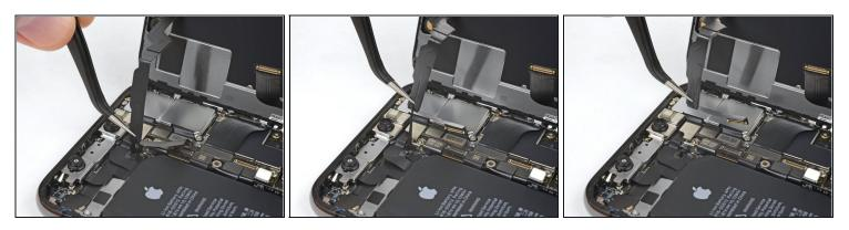
(i) The front panel sensor assembly flex cable is lightly adhered in place.
