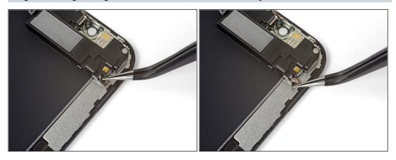
• On the back of the display assembly, peel back and remove any tape covering the hidden screw at the lower right corner of the speaker housing.
