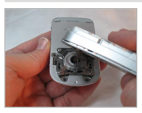
The back housing is now disassembled, and the swivel assembly is revealed.
