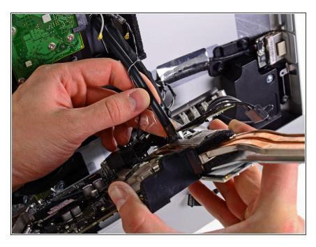
If present, peel off the tape securing the hard drive SATA cable to the logic board.
