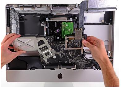
Slightly pull the logic board away from the back of the outer case, then lift it upward to clear the lower front face of the outer case.
