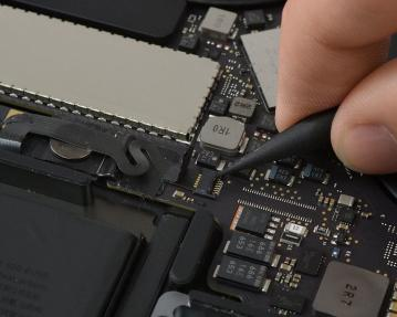
Use the tip of a spudger to flip up the small black locking tab securing the cable in its connector.
