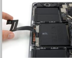
• Carefully peel the trackpad ribbon cable up off the battery, and push it out of the way.
