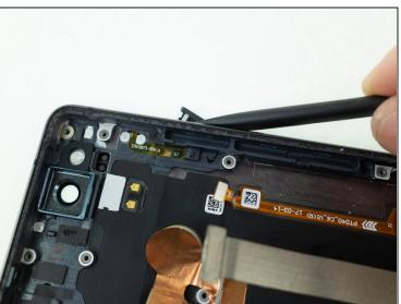
Push the external power and volume buttons out of the case with a spudger.
