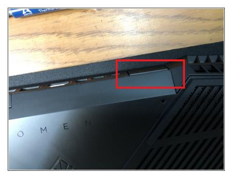
Grasp the back cover where the hinges are for the display. Pull upwards from the laptop, you will need to use some force the very fist time you open it.
