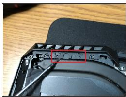
Remove the four screws from the cover. Insert a flathead screwdriver or a razor blade to lift the cover off the plastic nubs that hold it in place.
