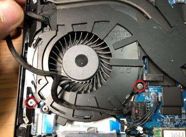
Remove the screws from the metal cover, lift away from the fan.
