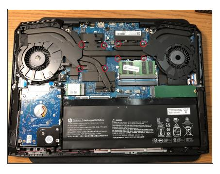
Remove the 8 screws holding the heatsink to the dies. Note that you need to remove the fan covers first.
