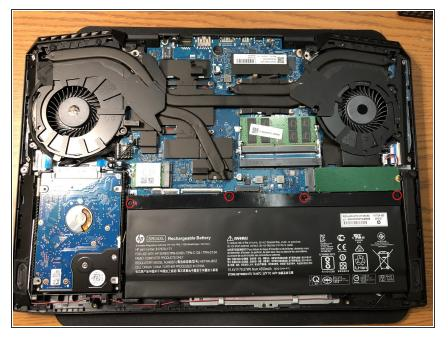
Remove the 4 screws holding the battery in place. Once removed, pull up on the plastic bar connected to the battery.
