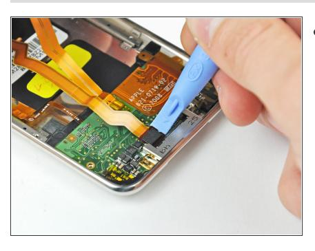
Use an iPod opening tool to pry the display cable connector up off its socket on the logic board.
