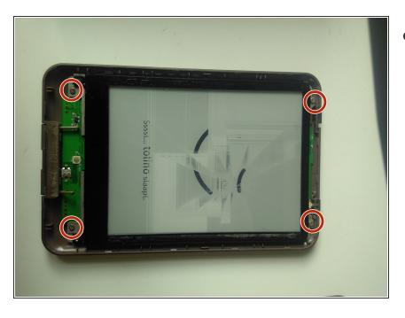
Remove the back cover by unscrewing the 4 screws indicated in red
