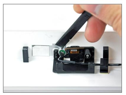
Use the flat end of a spudger to pry the microphone off the adhesive holding it to the front bezel.
