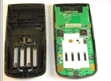
Pry back case off. Insert the plastic opening tool in the track for the protective cover and pry the halves of the case apart.
