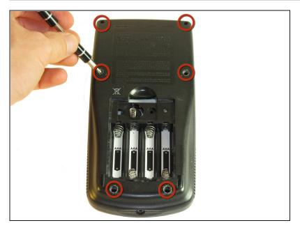
Unscrew the six 7.5mm T6 screws on the back case. You will need to use a screwdriver with a long and skinny head.
