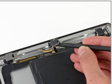
• Use the flat end of a spudger to pry the camera ribbon cable out of its socket in the plastic antenna housing.
