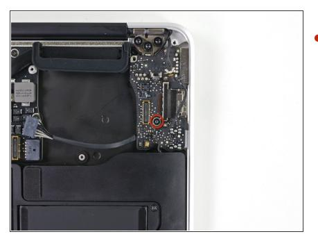
Remove the single 4.0 mm T5 Torx screw securing the I/O board to the upper case.
