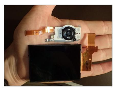
Remove rear control panel & display, threading ribbon cables through slot in camera body.
