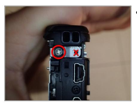
when replacing the top case, remember that the end screw goes on the right end of the camera (the screw hole on the left end is filled by one of the outer case screws). There are two screw holes on the right end - this screw goes in the hole on the left/closer to the rear of the camera (again, the other is for one of the outer case screws).
