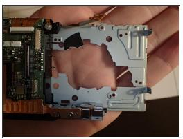
Turn camera over and remove lens assembly. This may take a bit of wiggling. Lift bottom right corner slightly, then pull lens assembly gently right and it will slide out.
