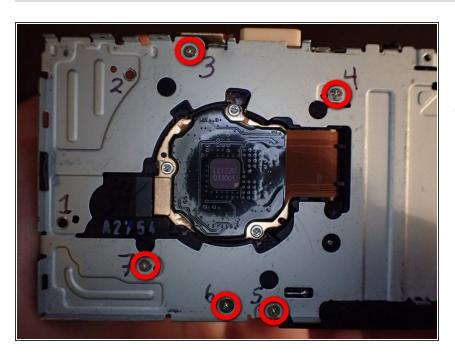
Remove remaining 5 numbered screws (3-7) from back of camera (numbers 5 & 6 are shorter than all the other numbered screws and different from each other; other numbered screws appear to be the same size, including 1 & 2).
