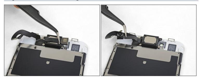
• Lift the front facing camera up out of its socket and swing it out of the way.
