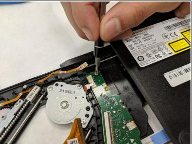
• Remove the single 3mm Phillips #0 screw to loosen the large circuit board.
