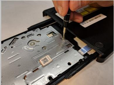
• Turn the unit over and remove the two silver 3mm Phillips #0 screws from the aluminum cover.
