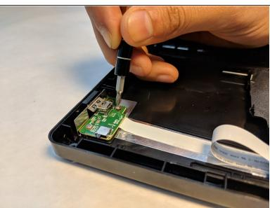
Remove the two silver 3mm Phillips #0 screws from the mini USB circuit board.
