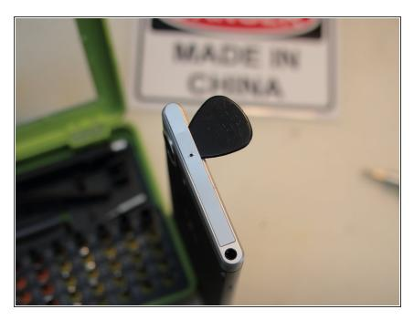
Carefully remove the top plastic cover. It is held in place by adhesive.
