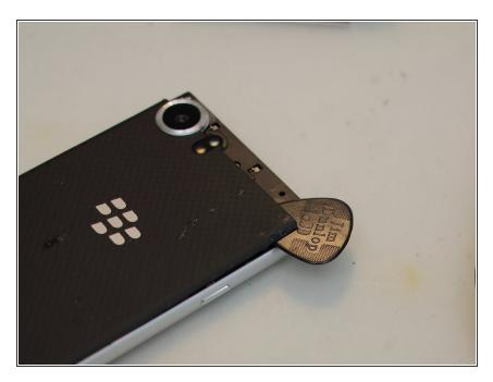
Remove the back cover. It mostly just clips off, but has some adhesive in the lower area.
