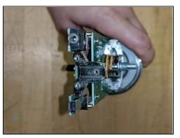
• On this step, you can easily and carefully pull the entire mic mechanism from the protective housing. On the bottom you will see where the Audio port and USB port are if you need to replace them.
