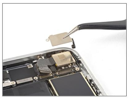
• Remove the rear-facing camera bracket.
