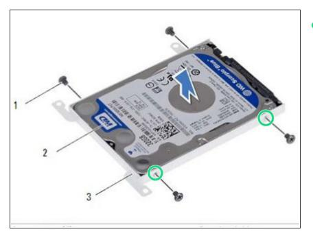
Align the screw holes on the harddrive bracket with the screw holes on the hard drive.
