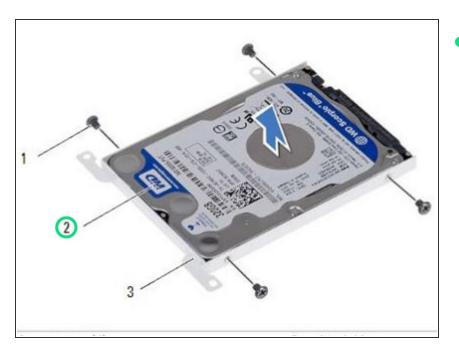
Place the NEW hard drive into the hard-drive bracket.
