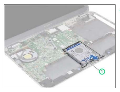
Place the hard-drive assembly on the computer base.
