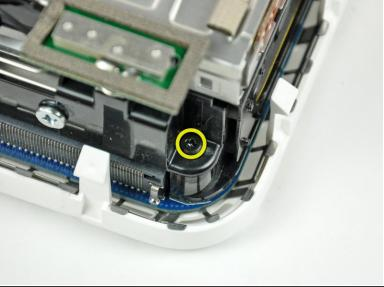
• Remove the Phillips screw from the internal frame near the Bluetooth antenna.
