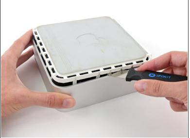
Keep working around the perimeter, freeing the clips along the final edge.
