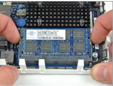
Simultaneously pull the tabs on each side of the RAM chip away from the center of the chip. These tabs lock the chip in place and releasing them will cause the chip to "pop" up.
