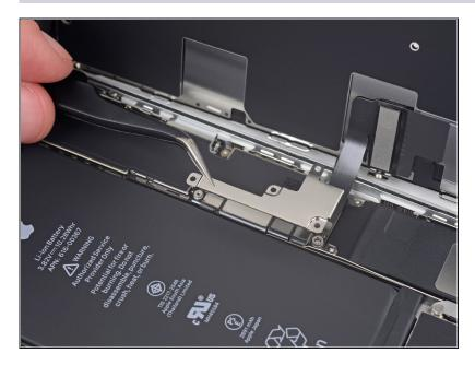
• Remove the lower display cable bracket.
