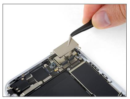
• Remove the cover plate from the rear camera module.
