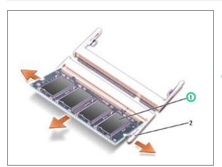
Slide the **NEW** module firmly into the slot at a 45-degree angle, and lower the module until it clicks into place. If
