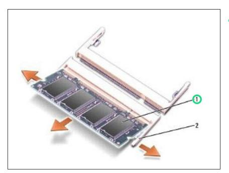
• Remove the module from the connector at a 45-degree angle.
